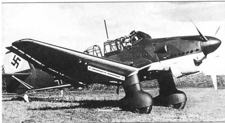
Above: A pre-production version of a Ju 87B-0. Note the extended air brakes below the wing.
