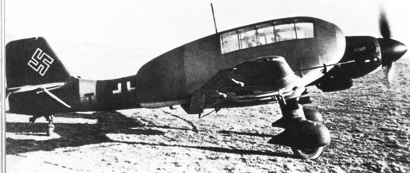
Above: A Ju 87D-3 variant, fitted with two storage pods attached to each wing. These types were very rare.
