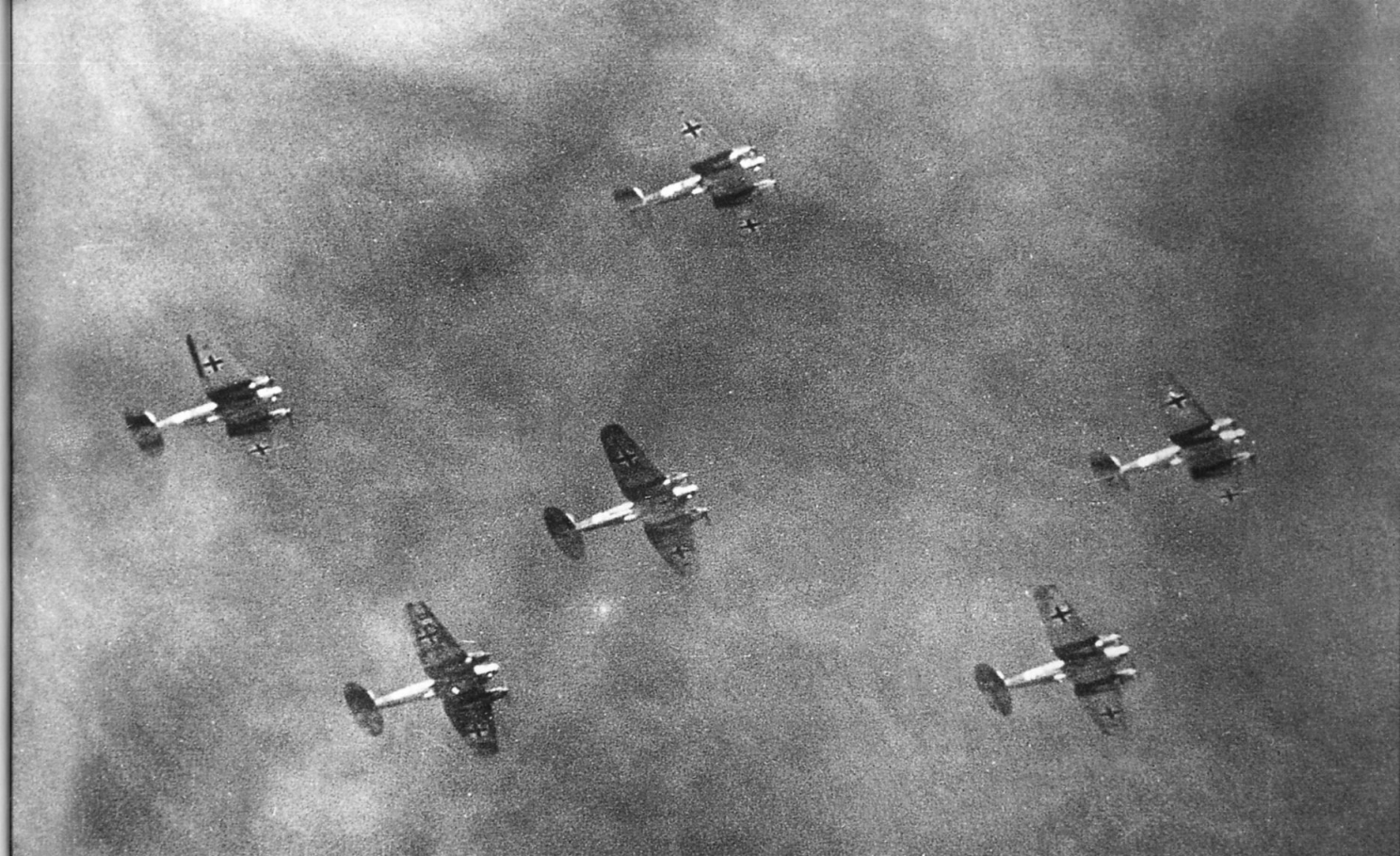
Above: German Heinkel He 111 medium bombers roar overhead on their way to bomb airfields during the Battle of Britain. Each aircraft was capable of carrying 2000kg (4410lb) of bombs up to a range of 1200km (745 miles).
