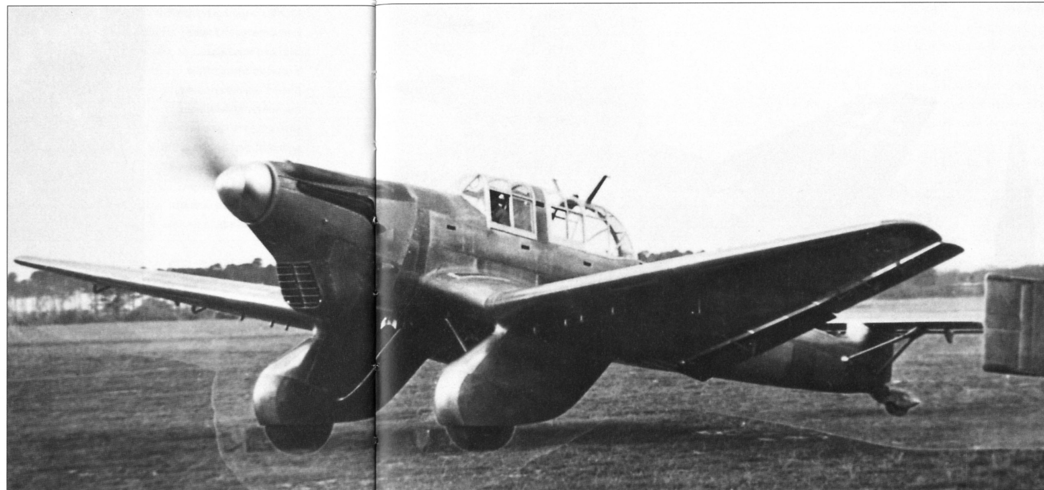
Above: The V-1 prototype version of the Ju 87 Stuka. The V-1 undertook its maiden flight on 17 September 1935. Note the double fin tail.
