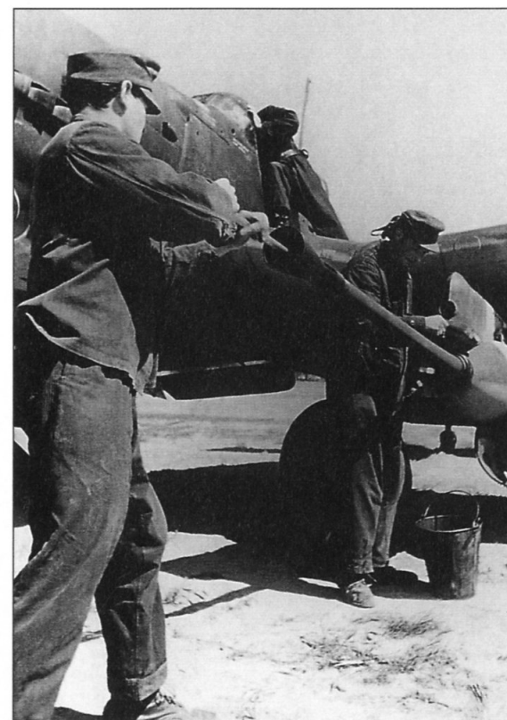
Above: Luftwaffe ground personnel perform essential maintenance on the 37mm anti-tank cannon of a Ju 87G Stuka on the Eastern Front, mid-1944.
